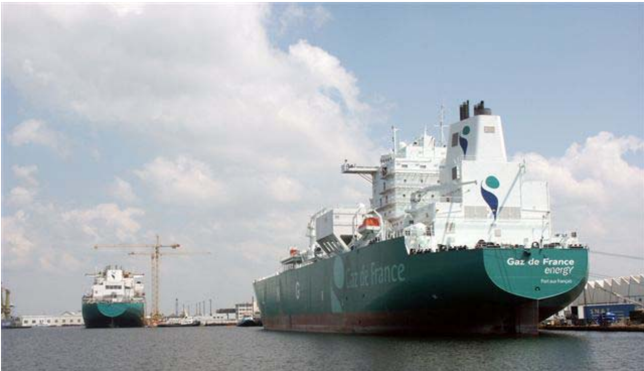
Figure 1: Liquefied natural gas today is increasingly being transported unpressurised at -163\text{ }^{\circ}\text{C} . (Photo: Rolf Müller-Wondorf)
