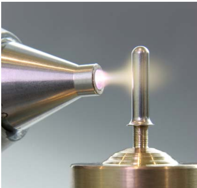
Ultrafine precleaning and activation in injection moulding technology. The metal pin is subsequently encapsulated in plastic.
