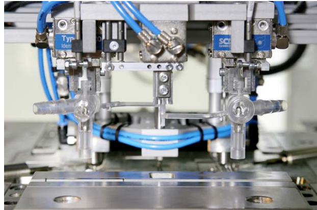
The finished components with the encapsulated metal insert are removed from the cavity in pairs.
