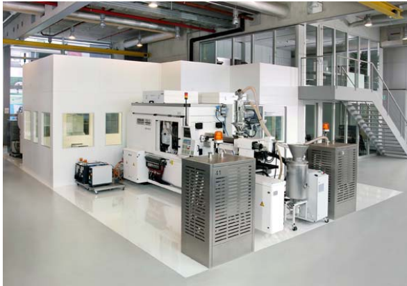
Stringent requirements in medical technology: The entire volume of air in the clean room is exchanged 80 times per hour.
