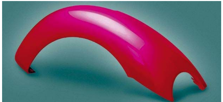
Fig. 5 Pretreatment with plasma ensure a flawless visual appearance of the painted surface.
