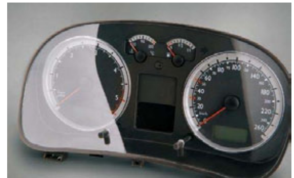
Fig. 6 After injection moulding but prior to painting of instrument module housings, there first ensues microfine cleaning with atmospheric-pressure plasma
