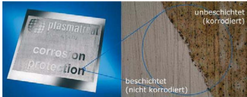
Fig. 8 Demonstration of the selective mode of action of a plasma polymer layer: the logo and inscription areas on an aluminium plate after 96 hour exposure to the salt spray test.
