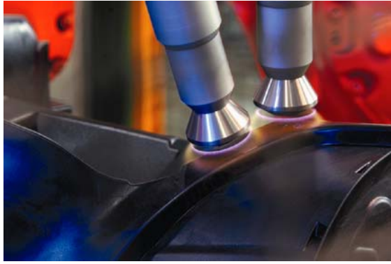
FIGURE 1 The atmospheric Openair plasma beam operates in a patterned manner and brings about microfine cleaning and strong activation of the polypropylene surface of the dashboard.
