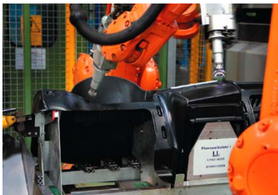
FIGURE 3 The plasma nozzles mounted to two robot arms pass over the surface true to contours and exactly keep those areas untreated where no PUR foam adhesion is desired.
