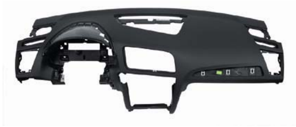
FIGURE 5 A milling system provides for the instrument openings. The back-foamed slush skin can be easily manually removed from the non-plasma-treated areas.
