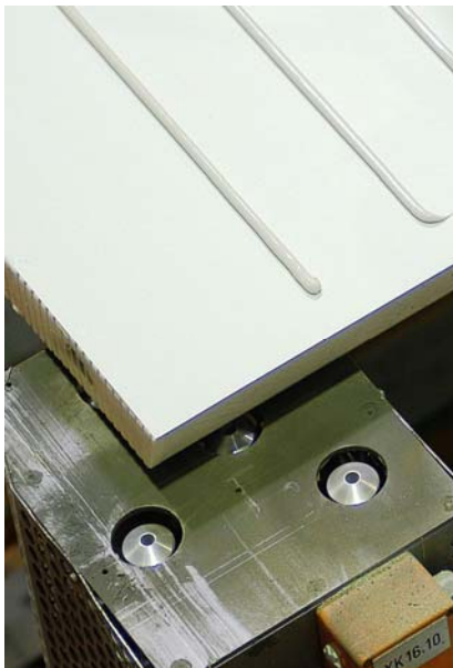
Adhesive bead application: The surface is cleaned to a microfine level and activated on a minimum width of 300 mm. Photo Plasmatreat
