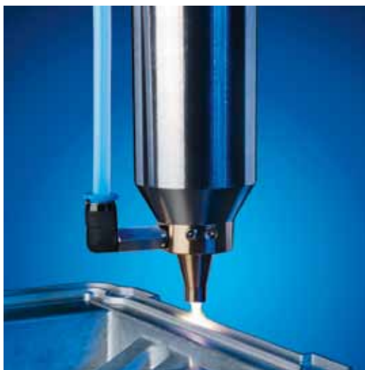
The anti-corrosive adhesion promoter layer provides not only a high corrosion protection, but is also a good tie coat for many adhesives
