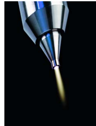
Figure 2 The electrically neutral Openair plasma beam allows microscopically fine cleaning, high activation and paper-thin coating of surfaces
