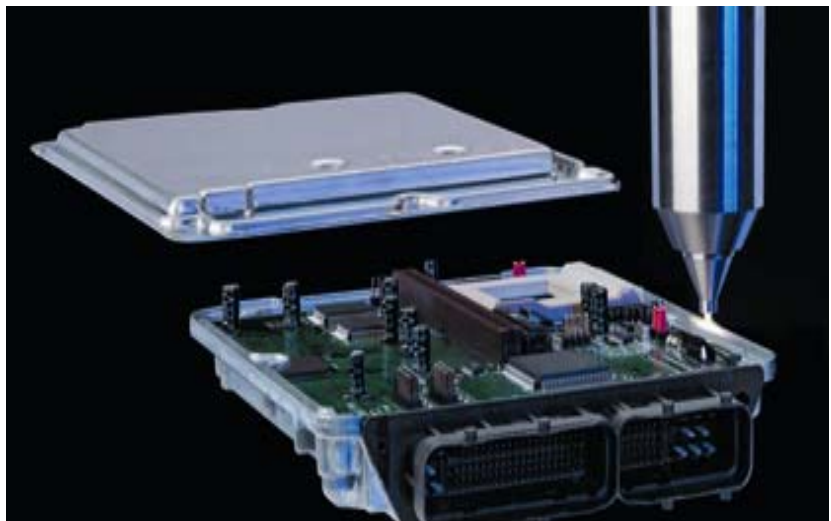
Photo: Plasmatreat The pretreatment and activation of the surfaces of housings prior to application of adhesive by Openair plasma brings about optimum imperviousness of the electronics
