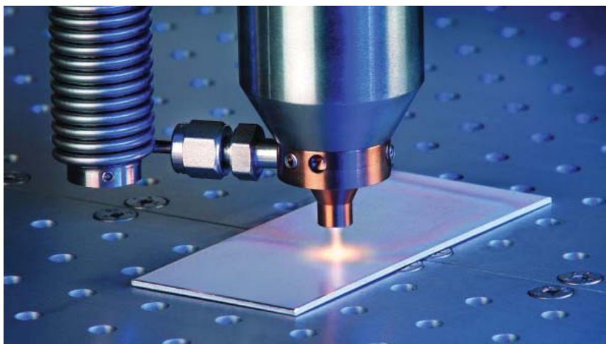
Photo: Plasmatreat Fig 1: No costly vacuum chamber needed: The new PlasmaPlus technology applies nanothin coatings to material surfaces under atmospheric pressure
