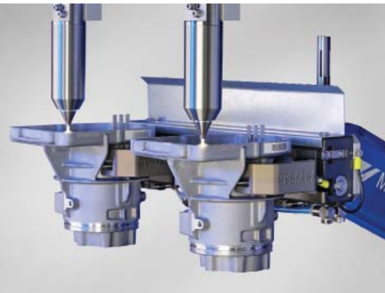
Photo: Plasmatreat Fig 3: TRW Automotive subjects the groove surfaces of engine pump housings to microfine cleaning and activation with an Openair plasma prior to PlasmaPlus coating
