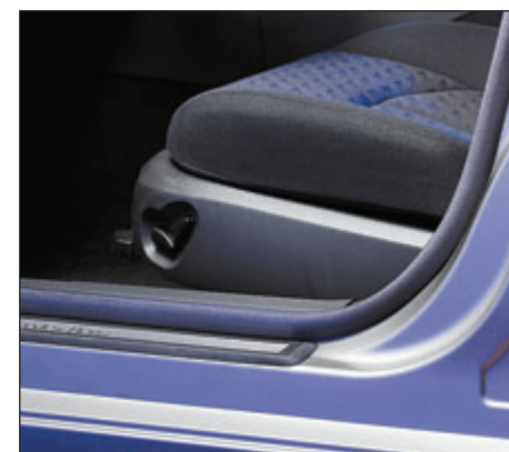
Fig. 5. Pretreatment with plasma allows for optimal bonding of the EPDM profile located in the door frame.
