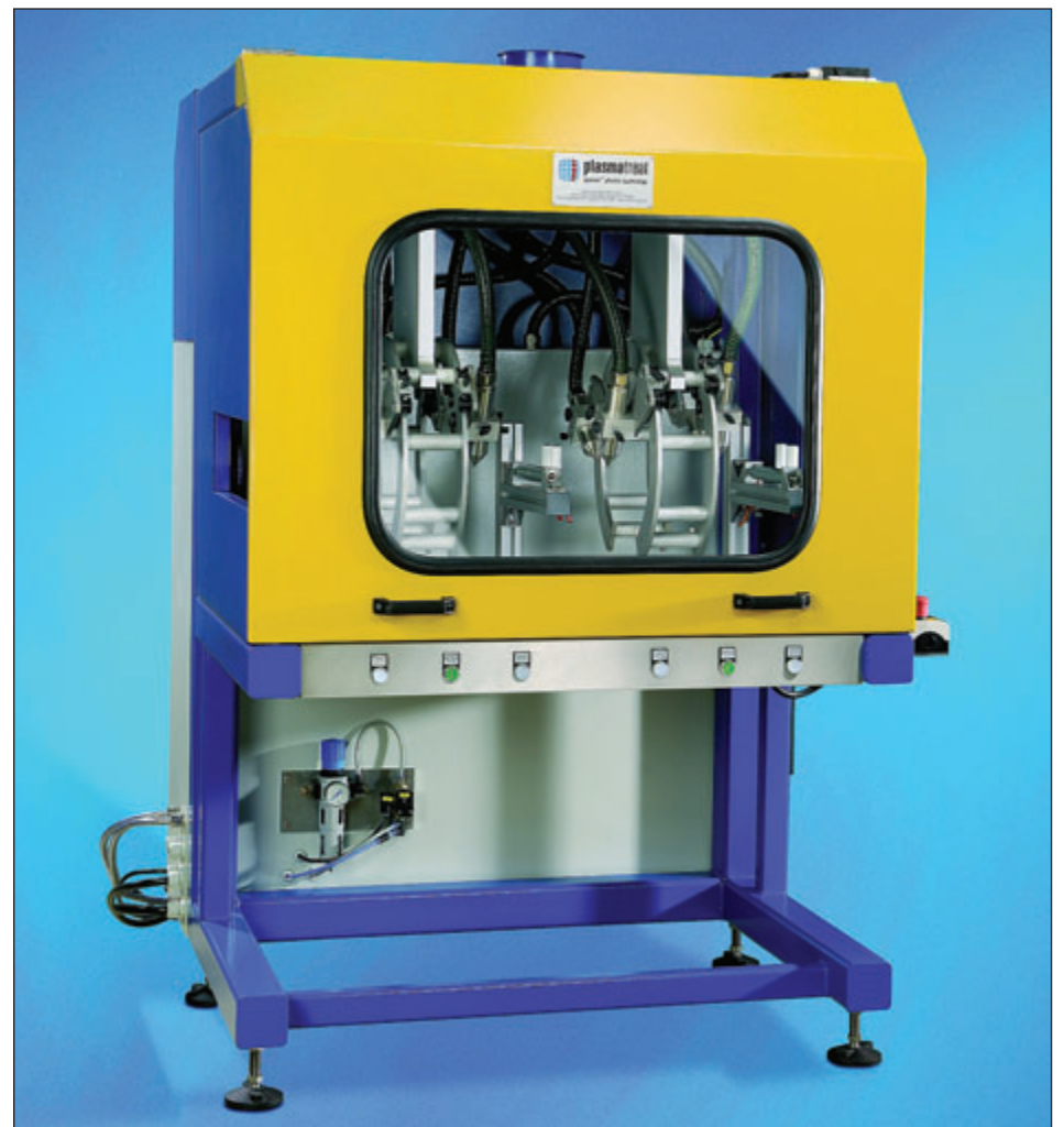
Fig. 8. Latest C-frame plasma treatment station. This particular model houses eight plasma jets.
