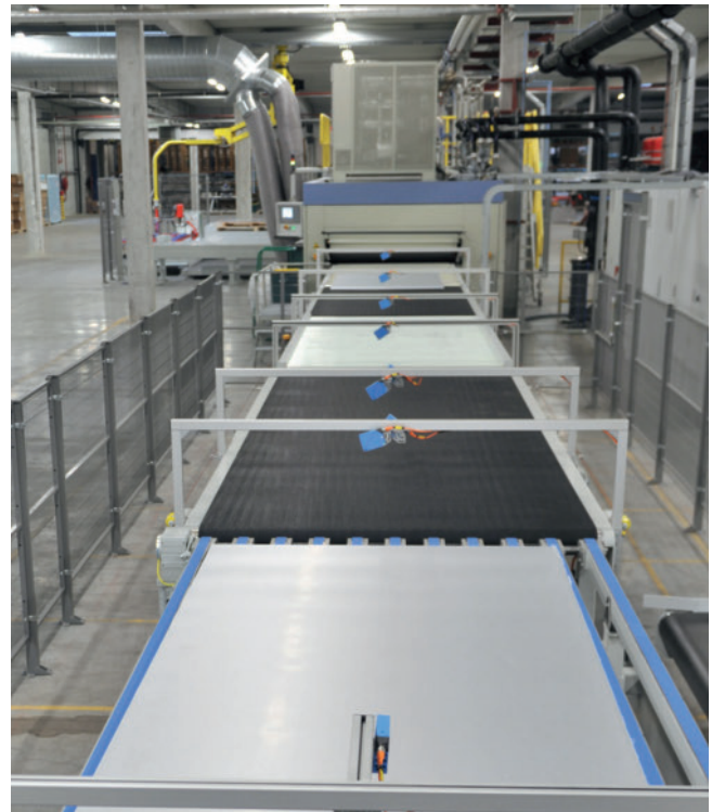
Fig. 8. The steel-faced honeycomb PP panels are manufactured at Elytra in a fully automatic production process (photo: Elytra)
