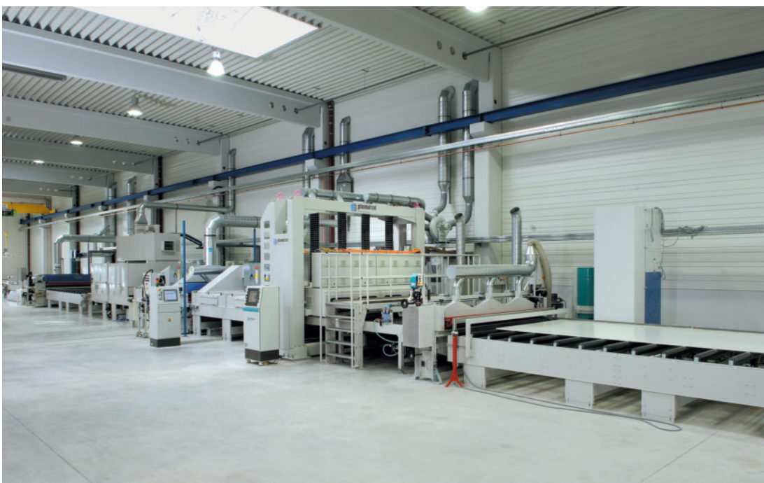
Fig. 2. The newly developed rotary nozzle system from Plasmatreat can pretreat sandwich panels up to approx. 3 m wide at a speed of 25 m/min in a continuous production process
