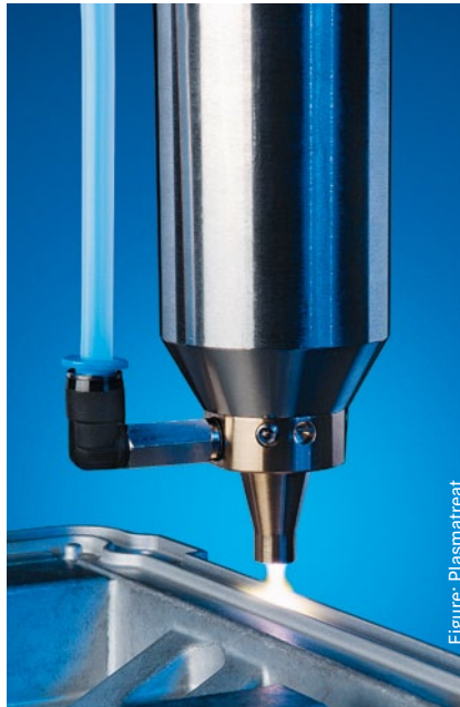
Figure 1: What was previously only achievable in the vacuum chamber is now possible in-line under normal atmospheric pressure: The functional coating of aluminium components.
