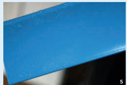
5 Wetting is far better after plasma activation (center) than after wet-chemical treatment.
