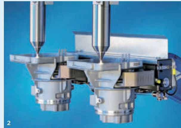
1 Functional coatings from the plasma nozzle: PlasmaPlus gives aluminum a high degree of corrosion protection.
