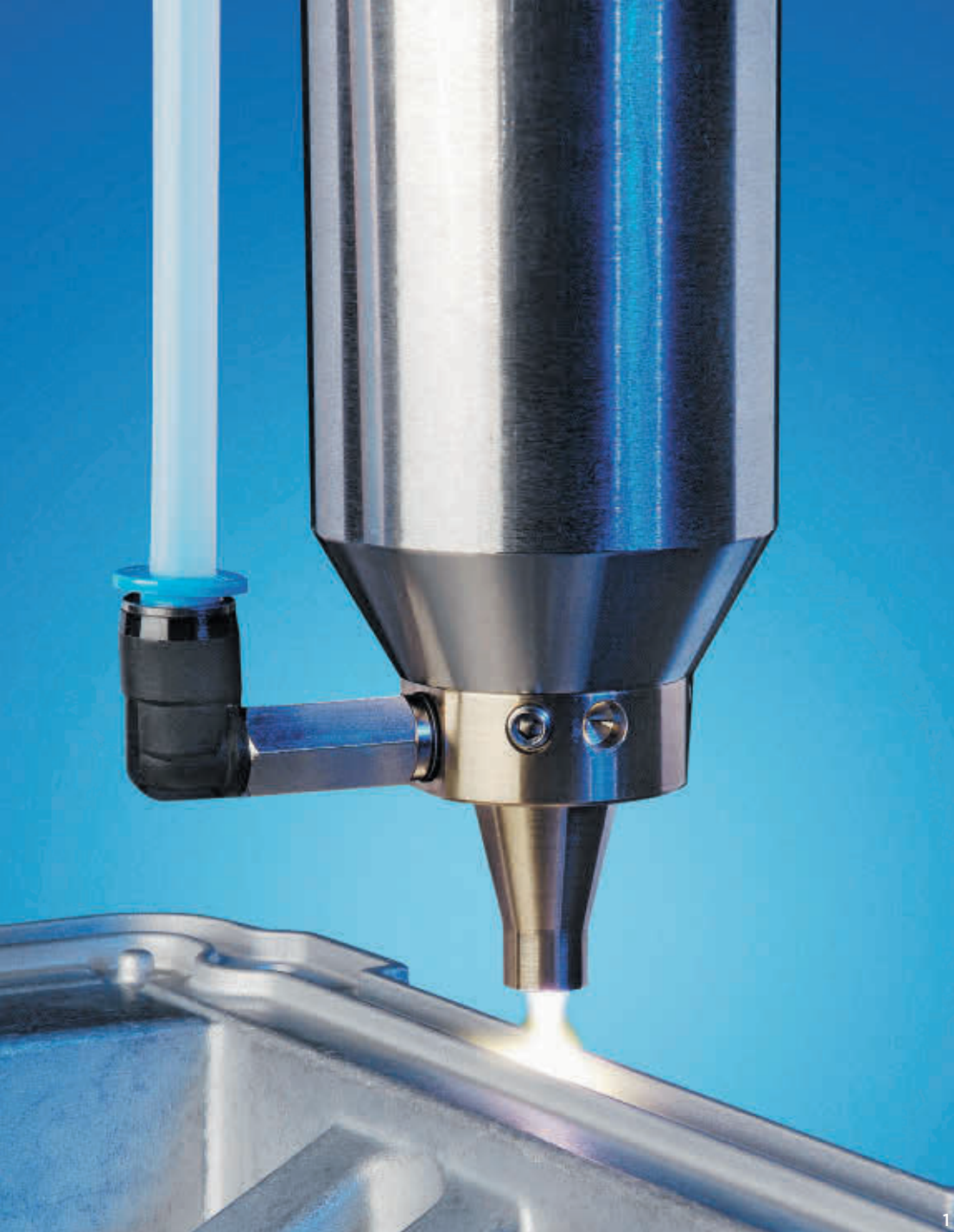
1 Functional coatings from the plasma nozzle: PlasmaPlus gives aluminum a high degree of corrosion protection.
