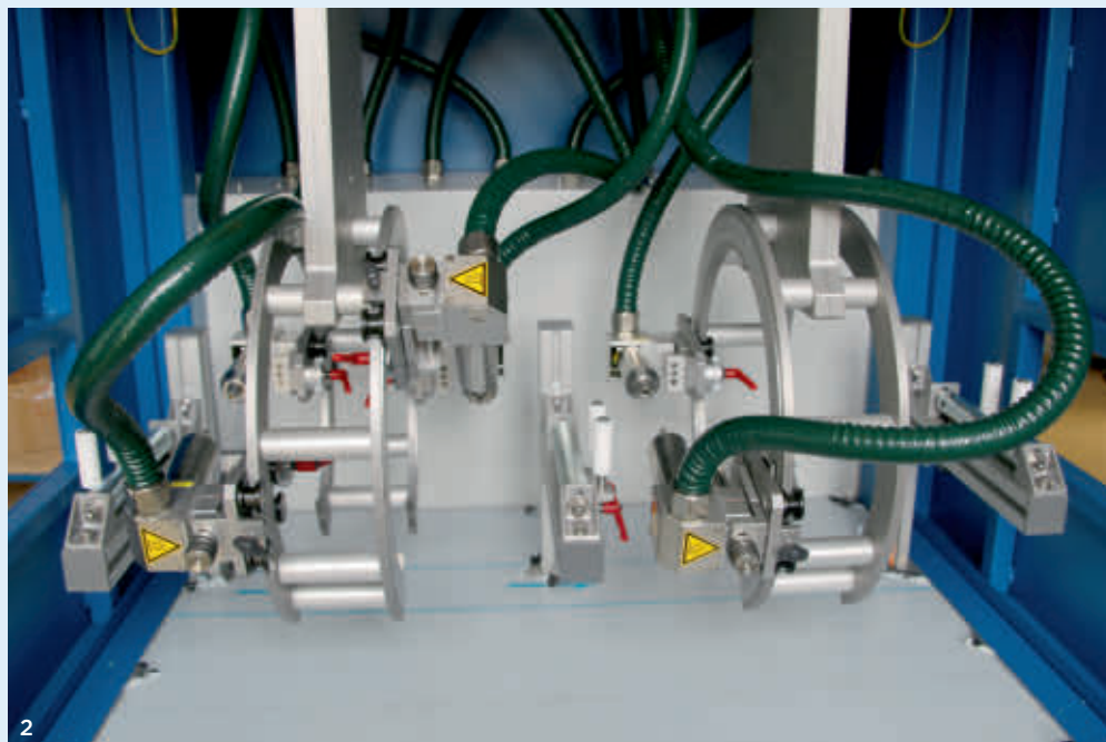
1 Mysterious: At this stage one can only imagine the numerous potential applications for plasma 2 The working chamber of an Openair plasma system for pipes and profiles
