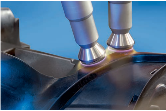
Fig. 3 > The robot-controlled plasma rotary nozzles carry out an area-selective treatment. By scanning the geometry of the instrument panel true-to-contour, they eliminate the need for masking before foaming.
