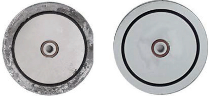
Fig. 4: Comparison of an uncoated AlSi12(Fe) die-cast aluminum test specimen (left) and one coated with the PlasmaPlus process after a 720-hour salt-spray test clearly demonstrates the benefits of the new technology (Photo Plasmamatreat)
