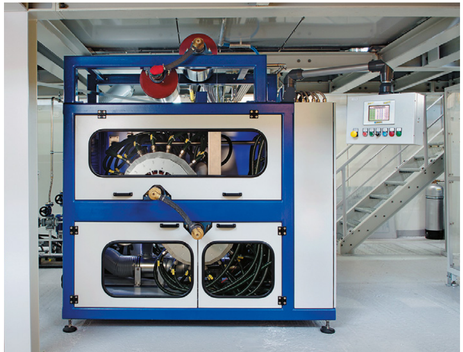
Fig. 5: With a footprint of just 2 m x 1.50 m, the computer-controlled plasma unit at Griesser brought about a fourfold increase in the production rate (Photo: Plasmamatreat)
