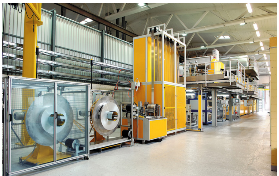
Fig. 2: The use of AP plasma on the new coating line installed by Griesser 12 years ago dispenses with the need for a wet-chemical cleaning line (Photo: Plasmatrete)
