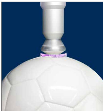
Openair-Plasma rotary nozzles work at speeds of 2700rpm. The plasma emitted at the side of the violet arc of light (not visible) strongly activates the surface of the ball, resulting in homogenous wettability. (Photo: Heidelberger Druckmaschinen AG)
