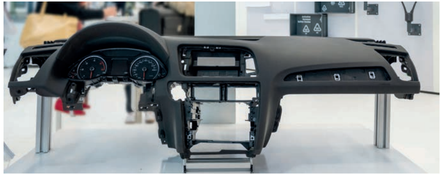
Fig. 4. The pretreatment with plasma makes non-polar plastics susceptible to adhesion processes and ensures a firm connection of the different, sometimes even incompatible materials, for example when laminating dashboards made of recycled materials with powder-sintered molded skins made of soft plastic. © Plasmatreteat
